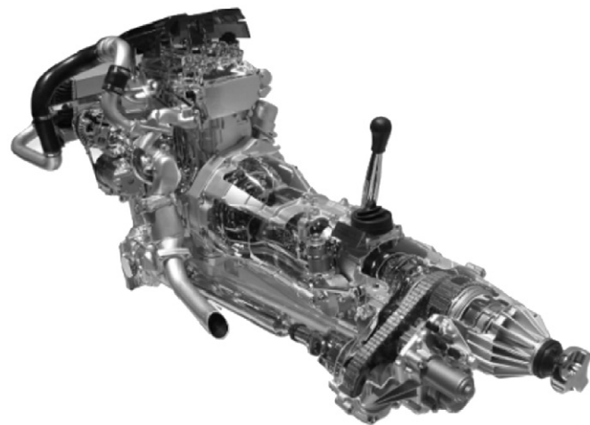
Fig. 12. The Nissan Pathfinder engine. It consists of 747 pieces and 330 parts.
