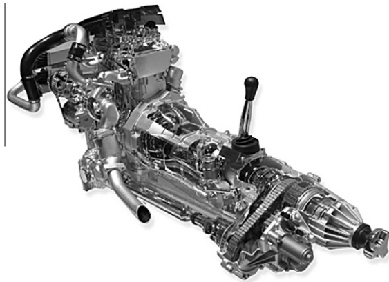
Fig. 10. The real engine of Nissan Pathfinder. It consists of 747 pieces and 330 parts.
